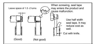
2. When installing piping or a joint, prevent contamination of chips or sealing agent. Also tightening torque should be within the range indicated below.
